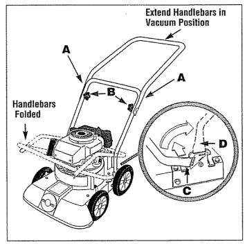
Figure 2: Handlebar position for vacuuming.
